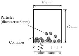
Fig. 3 Analytical model of the particle damper
