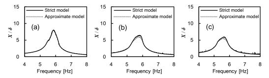
Fig. 11 Comparison of the calculation results between the strict DEM and approximate models. The time step is set to  $dt = 2.0 \times 10^{-5}$  s in the strict model, and  $dt = 1.0 \times 10^{-4}$  s in the approximate model. The number of particle is: (a) 20, (b) 40, and, (c) 60
