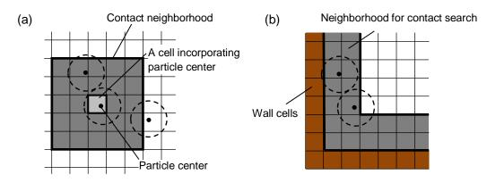
Fig. 6 Determination of collisions: (a) between particles, and (b) between particle and wall
