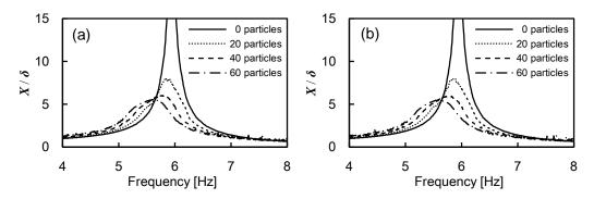
Fig. 9 Frequency responses of the particle damper calculated using the CA model. The twodimensional space consists of 32×20 cells. The unit time step is set to: (a)  $dt = 2.0 \times 10^{-5}$  s, and (b)  $dt = 1.0 \times 10^{-4}$  s
