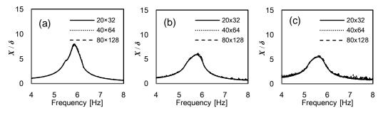
**Fig. 10** Effects of the two-dimensional space grid division on the precision of the frequency response calculation. The number of particle is: (a) 20, (b) 40, and, (c) 60
