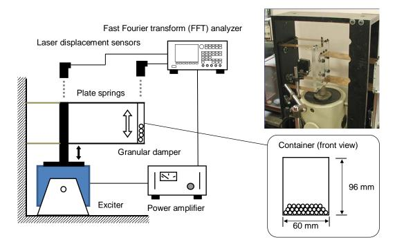
Fig. 1 Experimental setup of a vertically oriented granular damper
