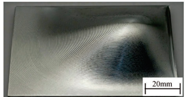
Fig.14 Machining result of free surface (order = 2, pitch = 0.2mm)
