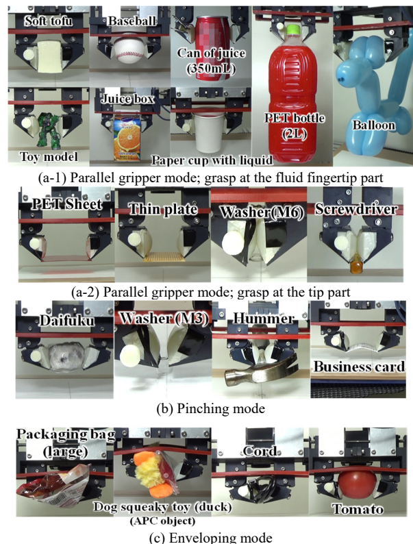
Figure 13. Representative results of grasping test
