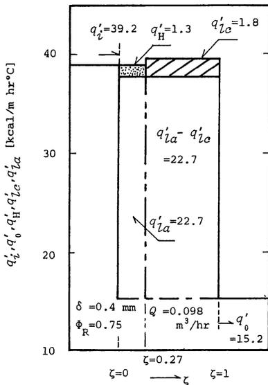
Fig. 11. Over-all Heat Balance of the Water Film for the case of  $\Phi_i > \Phi_R$  and  $0 < \zeta_R < 1$
