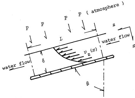
Fig. 2. Schematic representation of velocity profile of the falling water film
