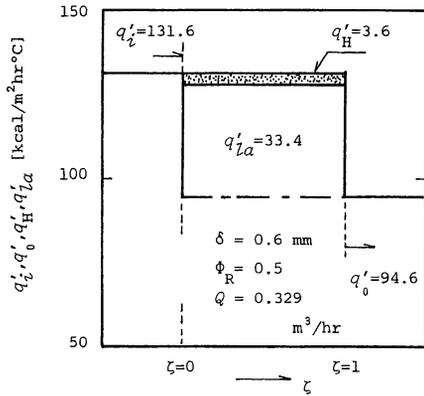
Fig. 10. Over-all Heat Balance of the Water Film for the case of  $\Phi_i > \Phi_R$  and  $\zeta_R > 1$  (where  $q'_{i0} = Q \rho C_p / LW$ ,  $q'_{o'} = Q \rho C_p \Phi_{av}(\zeta)_{\zeta=1} / LW$ ,  $q'_{La} = h_1 \bar{\Phi}(\xi)_{\xi=0}$ ,  $q'_{H'} = h_2 \{\bar{\Phi}(\xi)_{\xi=1} - \Phi_R\}$  and  $q'_{Lc} = h_2 \{\Phi_R - \bar{\Phi}(\xi)_{\xi=1}\}$ )
