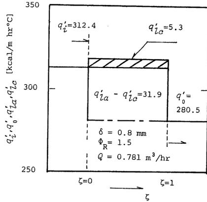
Fig. 12. Over-all Heat Balance of the Water Film for the case of  $\Phi_i < \Phi_R$
