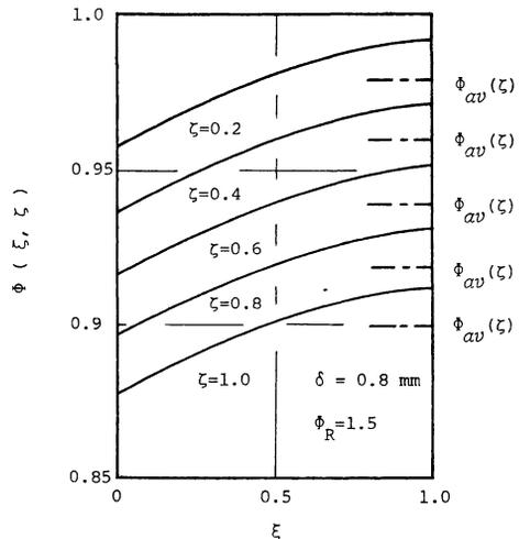
Fig. 7. Temperature profile of the falling water film for the case of  $\Phi_R=1.5$
