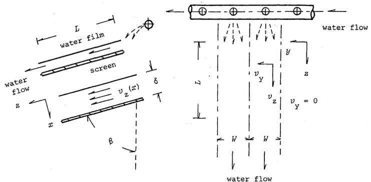
Fig. 1. Schematic representation of water spray and a falling water film on a screen
