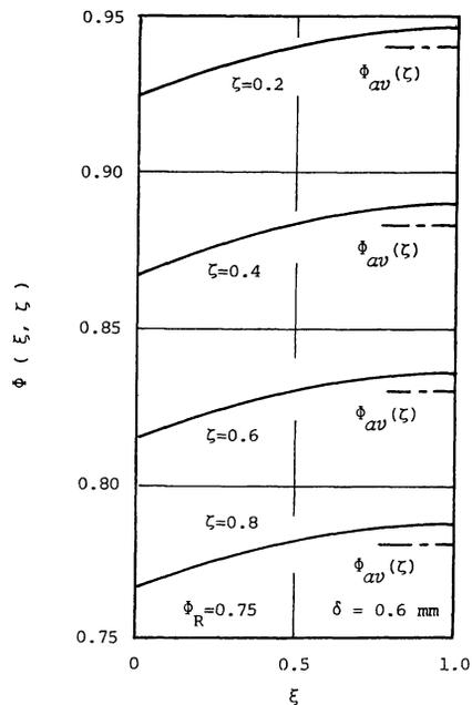
Fig. 4. Temperature profile of the falling hot water film
