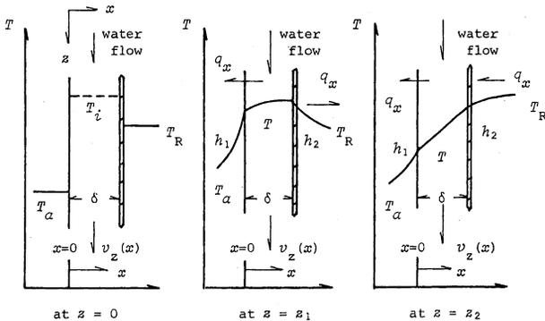
Fig. 3. Schematic representation of temperature profile of a falling hot water film
