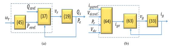
**Figure 3.** Control of DFIG: (a) rotor-side converter (RSC) controller; (b) grid side-converter (GSC) controller.
