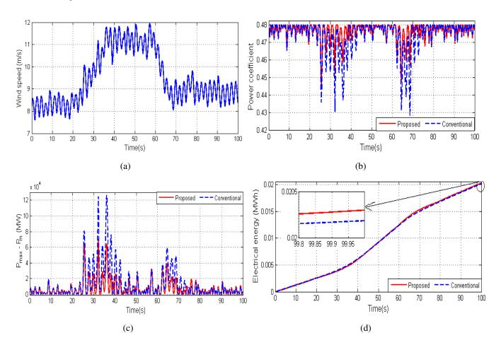
**Figure 9.** Simulation results with the rapid wind profile: (a) wind speed profile; (b) power coefficient; (c) error between  $P_{\text{max}}$  and  $P_m$ ; (d) electrical energy output.
