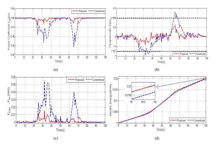
Figure 6. Simulation results using the proposed maximum mechanical power method: (a) power coefficient; (b) operation range of  $\lambda$ ; (c) error between  $P_{\text{max}}$  and  $P_m$ ; (d) electrical energy output.
