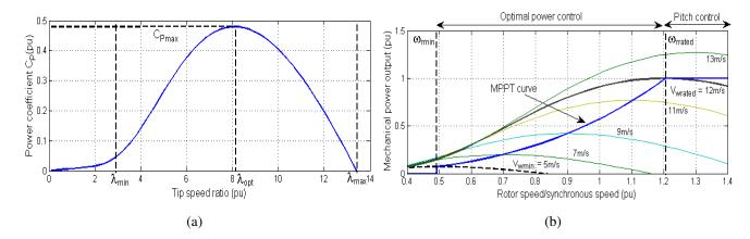
**Figure 2.** Characteristics of the wind turbine when  $\beta = 0$ : (a)  $C_p$  versus  $\lambda$ ; (b)  $P_{\text{max}}$  versus  $\omega_r$ .
