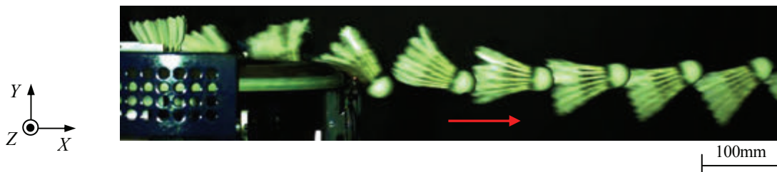
Fig. 16 For example, the flight behavior of the shuttlecock under the highest initial velocity is shown. This stroboscopic image is captured at every 1ms/frame using high-speed video. Initial velocity of the shuttlecock is 82.0 m/s.
