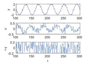
Fig. 3: A noisy case result of model-free predictive control using  $\ell_1$  minimization for the linear system (27). The variance of noise is four times larger than that in Fig. 2.
