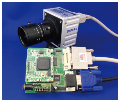
Fig.11 The developed emulation system composed of the high-speed camera and FPGA.
