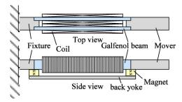
Fig. 1. Configuration of the device.
