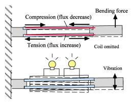
Fig. 2. Principle of energy harvesting (top: forces applied to Galfenol beams by bending force; bottom: electric energy generation by vibration).
