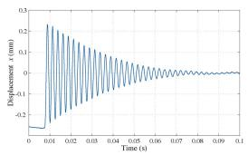
Fig. 6. Displacement at free vibration (fr = 392 Hz).
