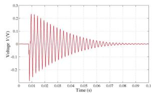
Fig. 5. Generated voltage at free vibration (fr = 392 Hz).
