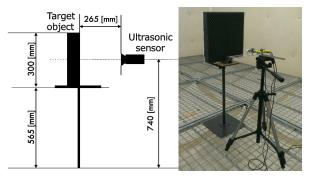
Figure 1. (left) Set-up of equipment and object, (right) In action (object: acoustic absorption material).
