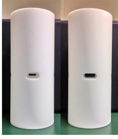
Fig. 11. The nozzle with uncovered holes.
