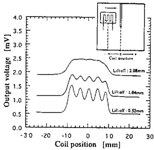
(a) Crack length parallel to the motion of the coil assembly
