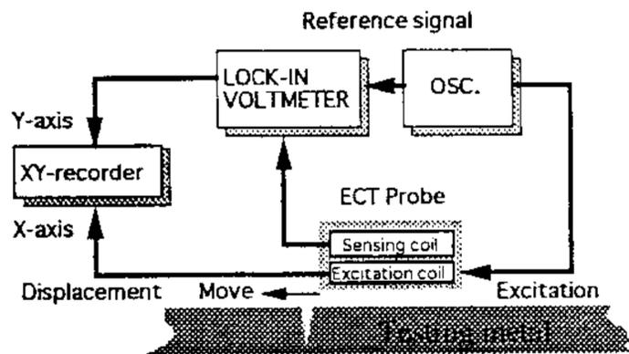
Fig. 4 Measurement System
