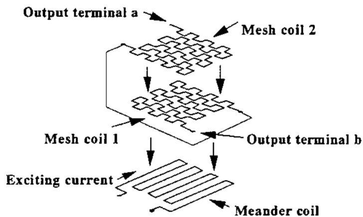
Fig. 8 Two Mesh Coil Configuration
