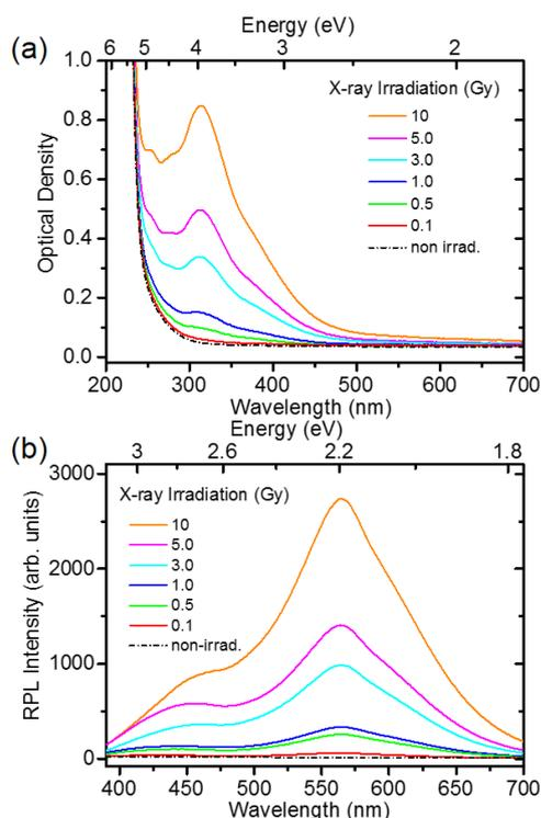
Figure 1. (a) OA spectra of Ag-activated phosphate glass with a thickness of 1 mm before and after X-ray irradiation with absorbed doses from 0.1 to 10 Gy. (b) Corresponding RPL spectra excited at 340 nm before and after X-ray irradiation at RT.
