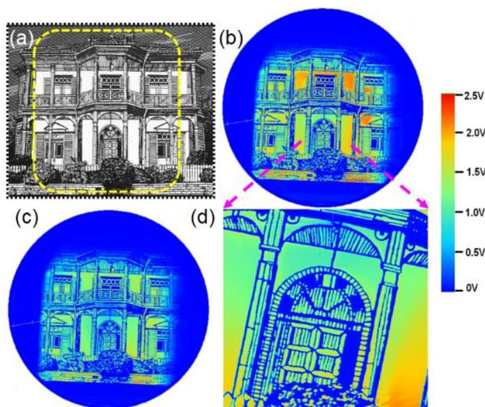
Figure 4. (a) Photo image of the mask used for X-ray irradiation. A set of reconstructed dose distributions acquired using the (b) orange and (c) blue RPL, respectively, and (d) an enlargement image of (b).
