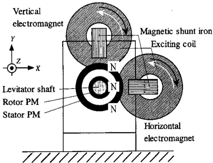
Fig. 3. Side view of the passive magnetic levitation unit seen from the symmetry plane. Two electromagnets are configured with the phase difference of 90 degrees in space.
