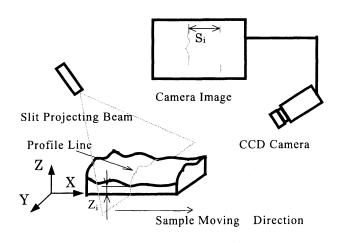
Fig.1 Schematic diagram of 3D measurement system
