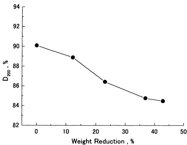
Fig. 9 Changes of revolving drap coefficient at 200 rpm with the weight reduction ratio for Kuraray fabrics.
