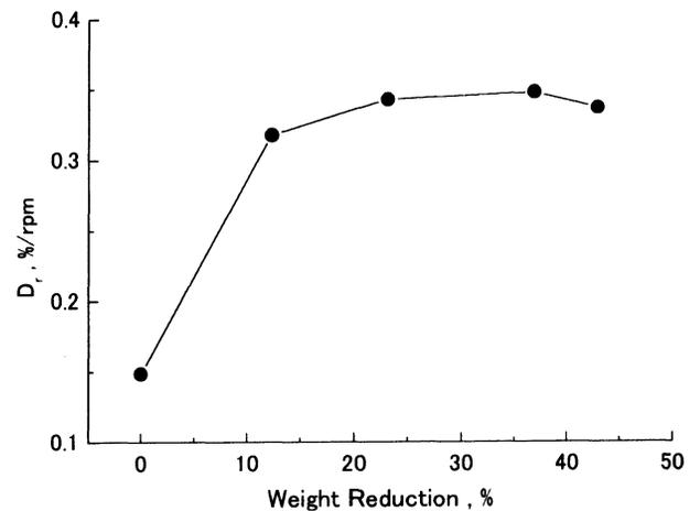
Fig. 7 Changes of revolving drape increase coefficient with the weight reduction ratio for Kuraray fabrics.
