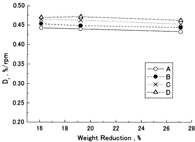
Fig. 8 Changes of revolving drap increase coefficient with the weight reduction ratio for Teijin fabrics.
