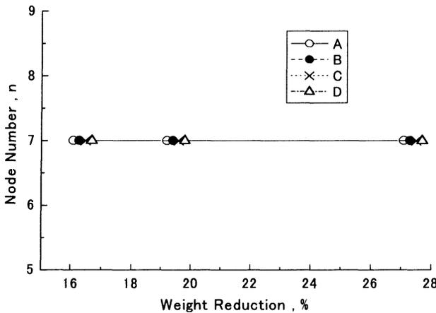
Fig.4 Changes of node number with the weight reduction ratio for Teijin fabrics.
