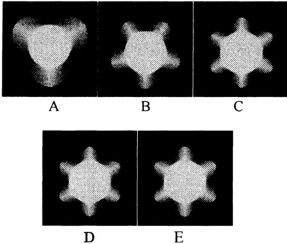
Fig. 3 Simulated models of fabric drape shapes for Kuraray fabrics with the weight reduction ratios: A;0%, B;12.3%, C;23.1%, D;36.9%, E;42.9%.
