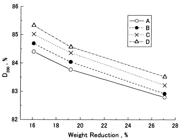
Fig. 10 Changes of revolving drap coefficient at 200 rpm with the weight reduction ratio for Teijin fabrics.
