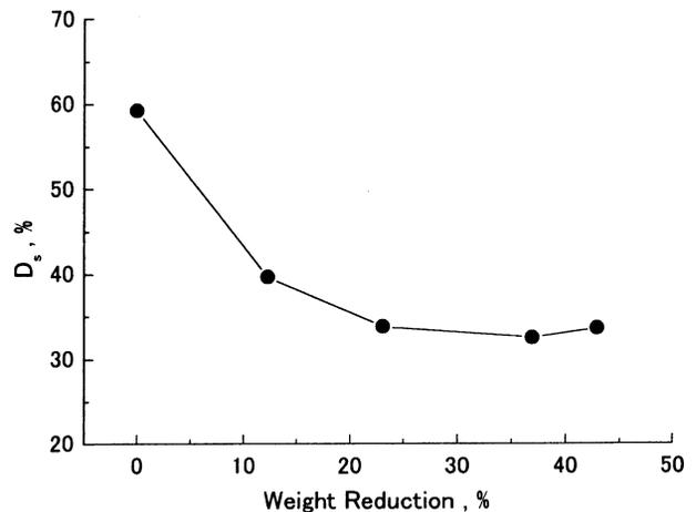
Fig.2 Changes of conventional static drape coefficient with the weight reduction ratio for Kuraray fabrics.
