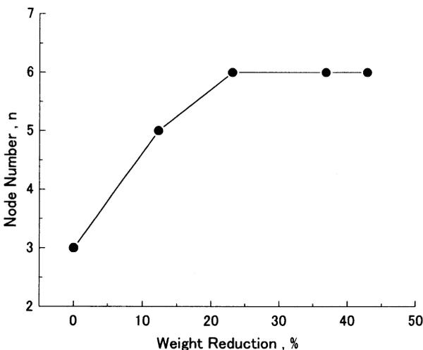
Fig.1 Changes of node number with the weight reduction ratio for Kuraray fabrics.
