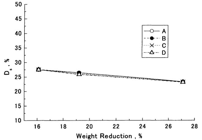
Fig.5 Changes of conventional static drape coefficient with the weight reduction ratio for Teijin fabrics.
