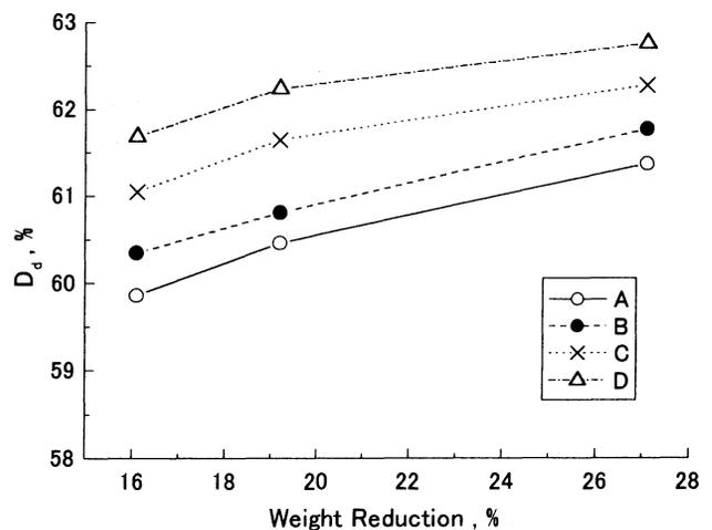
Fig. 12 Changes of dynamic drap coefficient with the weight reduction ratio for Teijin fabrics.
