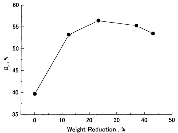
Fig. 11 Changes of dynamic drap coefficient with the weight reduction ratio for Kuraray fabrics.
