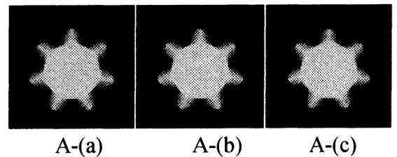
Fig.6 Simulated model of fabric drape shapes for Teijin fabrics with the weight reduction ratios: (a); 16.1%, (b); 19.2%, (c); 27.1%
