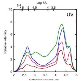
Fig. 2 Temperature-dependence of chromatogram of extracts from wheat bran with [C<sub>2</sub>mim][(MeO)(H)PO<sub>2</sub>] upper: with RI detector, lower: with UV detector.
