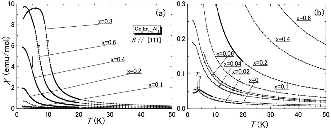
**Fig. 2.** (a) Temperature dependence of dc susceptibility  $\chi(T)$  for  $\text{Ce}_{1-x}\text{Er}_x\text{Al}_2$ . The arrow shows the inflection point which corresponds to the ferromagnetic temperature  $T_C$ . (b) The expanded scale of  $\chi(T)$  below  $x \leq 0.1$ . The arrow shows the antiferromagnetic temperature  $T_N$ .
