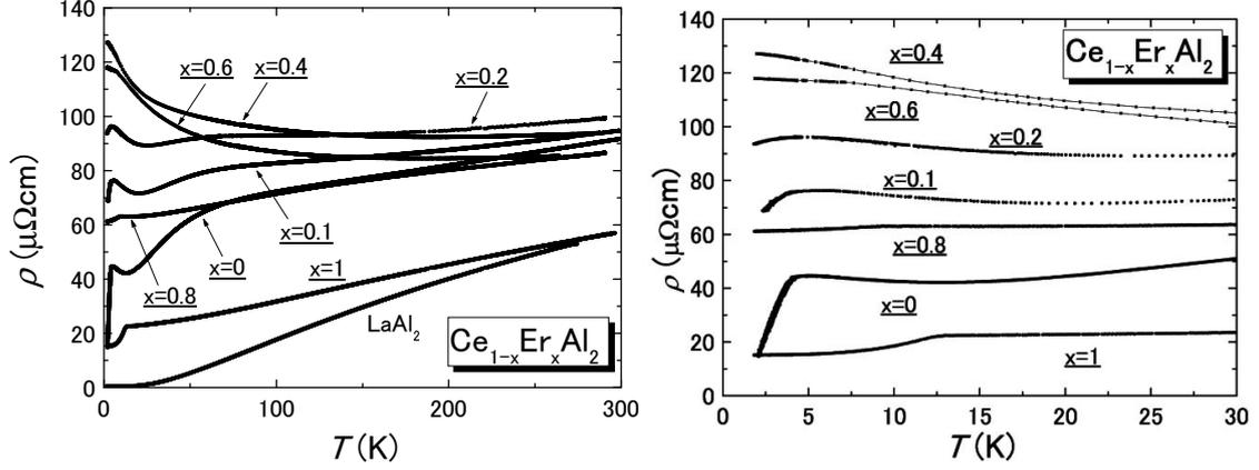
**Fig. 1.** Temperature dependence of the electrical resistivity  $\rho(T)$  in  $\text{Ce}_{1-x}\text{Er}_x\text{Al}_2$ . Right plot shows the expanded scale of  $\rho(T)$  below 30 K
