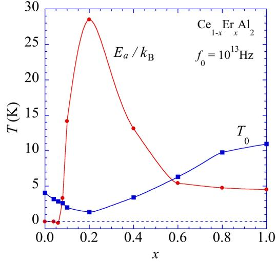
**Fig. 5.** The activation energy  $E_a$  and the Vogel-Fulcher temperature  $T_0$  obtained from fitting of freezing temperatures using the Vogel-Fulcher law.
