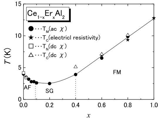
**Fig. 6.** Schematic phase diagram of  $\text{Ce}_{1-x}\text{Er}_x\text{Al}_2$  systems.
