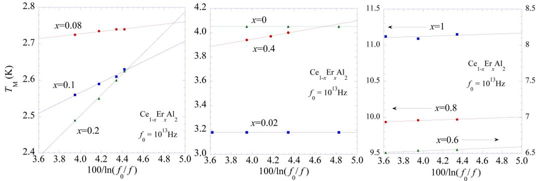
**Fig. 4.** Plot of  $T_M$  vs  $100/\ln(f_0/f)$  in the  $\text{Ce}_{1-x}\text{Er}_x\text{Al}_2$  series. The solid line is the least-squares fit of Equation (2). The  $f_0$  parameter was fixed at the value of  $10^{13}$  Hz. The obtained parameters are summarized in Fig. 5.
