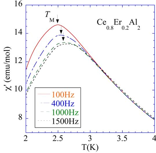
**Fig. 3.** Temperature dependence of ac susceptibility  $\chi'$  of  $\text{Ce}_{0.8}\text{Er}_{0.2}\text{Al}_2$  for several frequencies.
