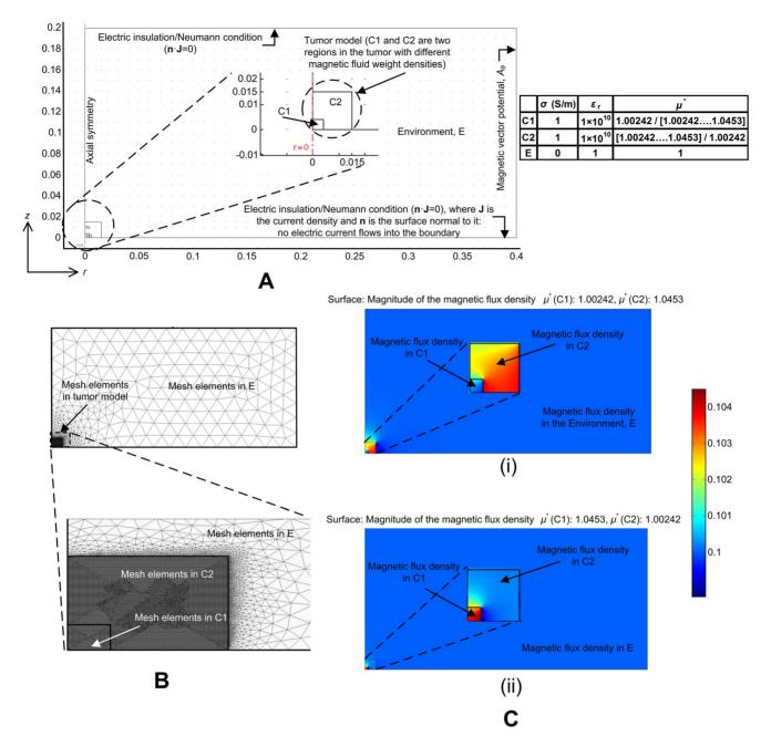
**Figure 2. Numerical modeling.** (A) 2-D, axial-symmetric model, (B) meshed model, and (C) solved model for the cases (i)  $D_{wi} < D_{wo}$  and ii)  $D_{wi} > D_{wo}$ . doi:10.1371/journal.pone.0081227.g002
