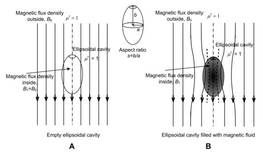
**Figure 1. Analytical model for estimating magnetic fluid weight density inside a tumor.** Magnetic flux density inside and outside a magnetic fluid-filled ellipsoidal cavity. The flux lines pass through the empty cavity (A) but converge in the cavity with magnetic fluid (B), thus leading to a difference in the magnetic flux density inside and outside the cavity. doi:10.1371/journal.pone.0081227.q001
