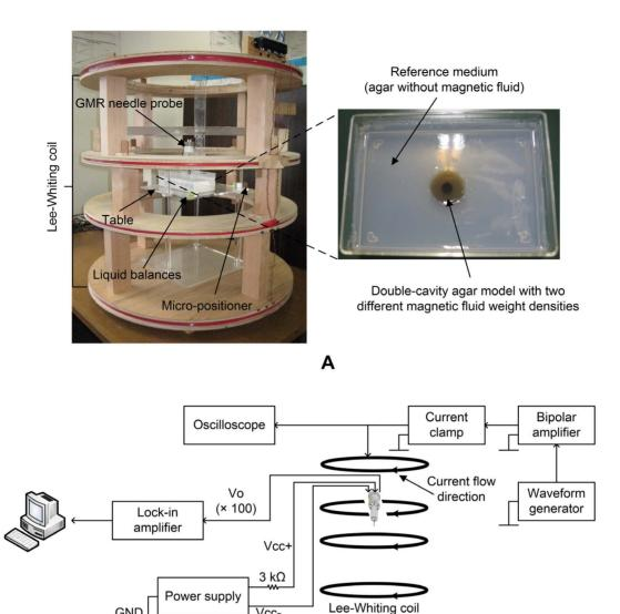
Figure 5. (A) Experimental setup, and (B) schematic of the data analysis setup. doi:10.1371/journal.pone.0081227.g005
