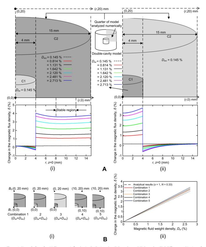
**Figure 6. Numerical results.** (A) The magnetic flux density distribution when (i)  $D_{wi} < D_{wor}$  and (ii)  $D_{wi} > D_{wo}$ . (B) (i) Different combinations of magnetic fluid weight densities to be estimated and surrounding media with varying weight densities. (ii) Comparison of magnetic fluid weight densities for surrounding mediums with different weight densities. doi:10.1371/journal.pone.0081227.q006
