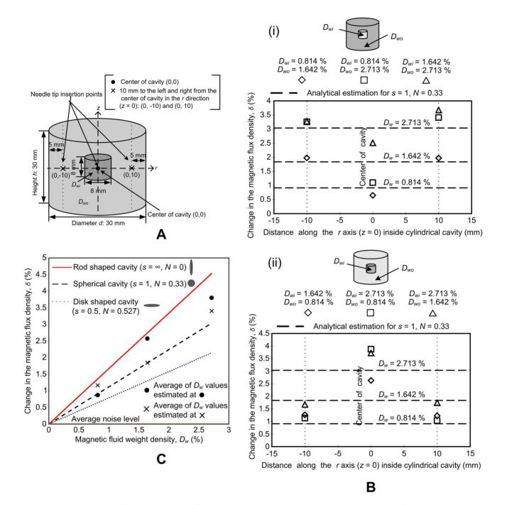
**Figure 8. Experimental analysis.** (A) Schematic of the double-cavity cylindrical agar tumor model. (B) Magnetic fluid distribution analysis in double-cavity agar models. (i)  $D_{wi} < D_{wo}$  and (ii)  $D_{wi} > D_{wo}$ . (C) Correlation of experimental data with analytical results. doi:10.1371/journal.pone.0081227.q008
