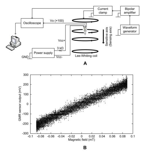
Figure 7. GMR probe characterization. (A) Experimental setup for characterization, (B) small-signal AC sensitivity at 100 Hz. doi:10.1371/journal.pone.0081227.g007
