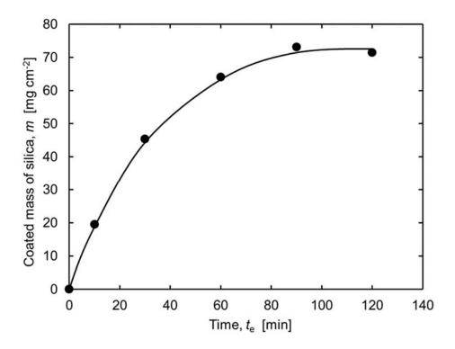
**Fig. SM-2** Effect of electrophoretic deposition time on coated mass of silica on aluminum (silica-sol solution of pH 10.6 with SDS of 0.05 mass%,  $V_e = 200$  V,  $T_e = 25^{\circ}$ C; aging treatment at 100 V for 5 h in ammonia water of pH 9.0).
