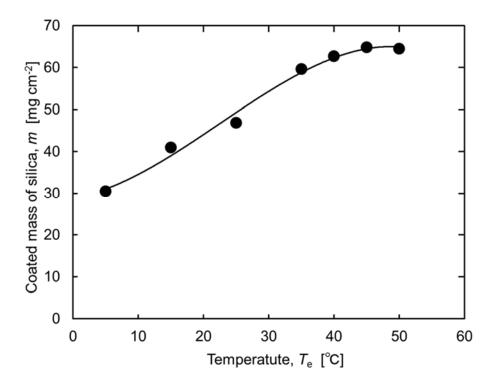
**Fig. SM-3** Effect of temperature of electrophoresis bath on coated mass of silica on aluminum (silicasol solution of pH 10.6 with SDS of 0.05 mass%,  $V_e = 200$  V,  $t_e = 30$  min; aging treatment at 100 V for 5 h in ammonia water of pH 9.0).
