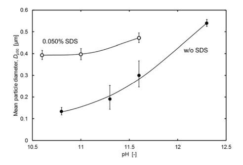
Fig.4. Relationships between mean diameter of silica particles and pH of silica-sol solution with and without SDS.
