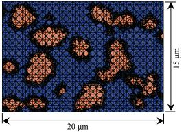
Figure 1 Finite element mesh created from micrograph
