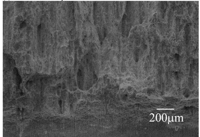
(b) SEM micrograph of SM490 fracture surface
