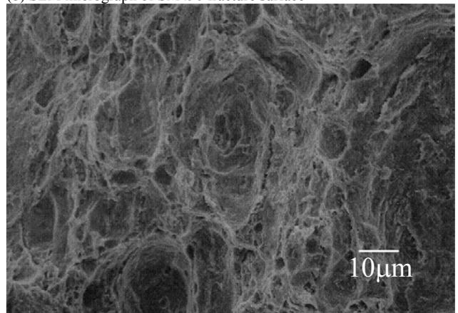
(c) SEM micrograph of SM490 fracture surface
