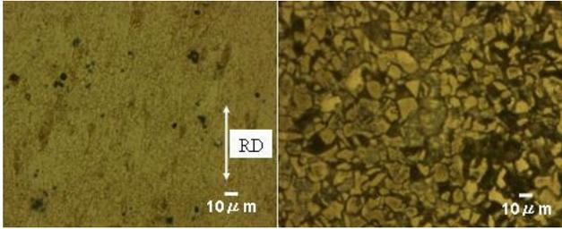
(a) NFG600, grain diameter ≈ 5 μm (b) SM490, grain diameter ≈ 15 μm
