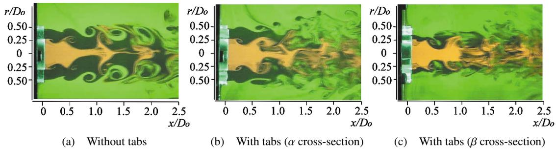
Fig. 11 Visualized flow patterns at  $x$ - $r$  cross-sections for the excited jet
