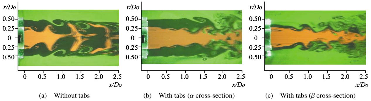
Fig. 4 Visualized flow patterns in  $x$ - $r$  cross-sections for the unexcited jet
