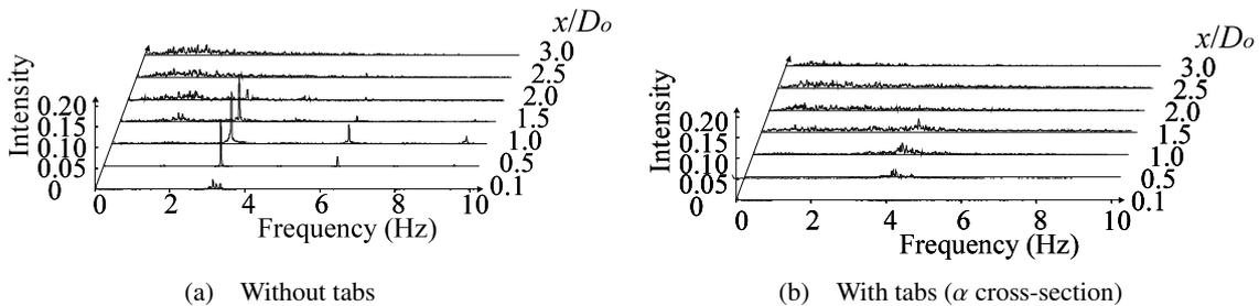
Fig. 10 Streamwise variation in velocity fluctuation signal spectra for the unexcited jet ( $r/D_o = 0.25$ )
