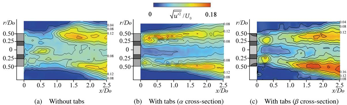
Fig. 8 Contours of streamwise velocity fluctuation RMS values for the unexcited jet
