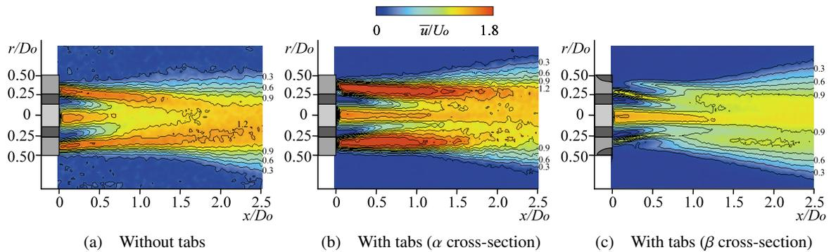
Fig. 6 Mean axial velocity contours for the unexcited jet
