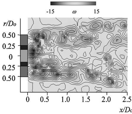
Fig. 15 Instantaneous vorticity contours for the excited jet with tabs at an  $\alpha$  cross-section
