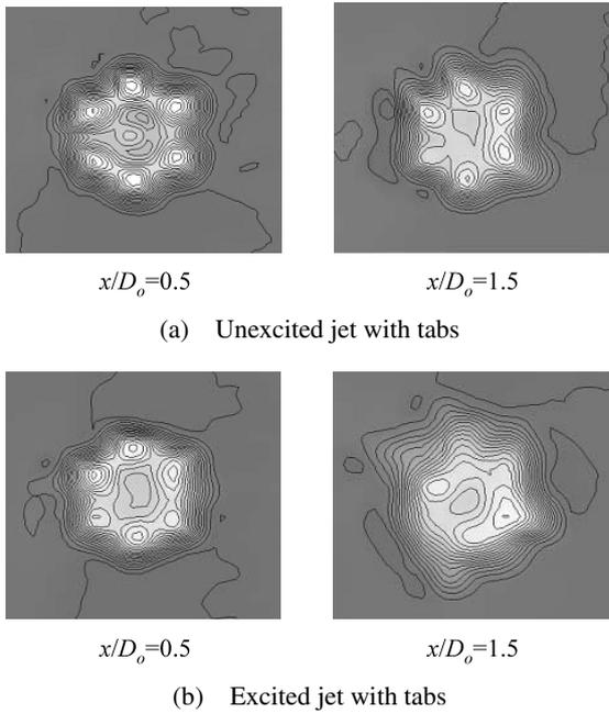
Fig. 16 Mean axial velocity contours at  $r$ - $\theta$  cross sections
