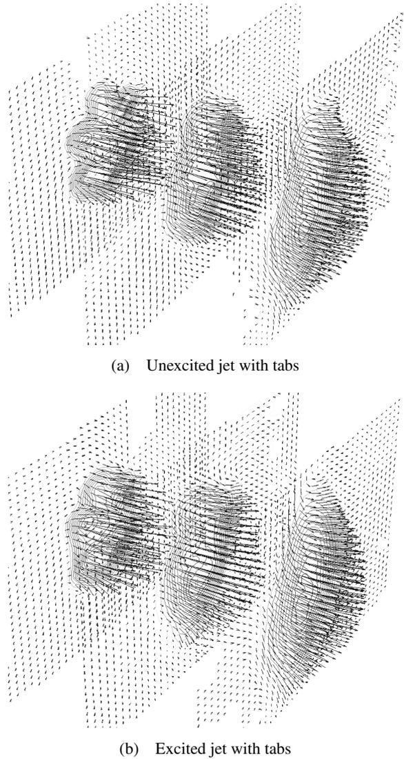
Fig. 17 Three-dimensional velocity vectors at  $x/D_o = 0.5, 1.5$  and  $2.5$  cross-sections for the tabbed coaxial jet
