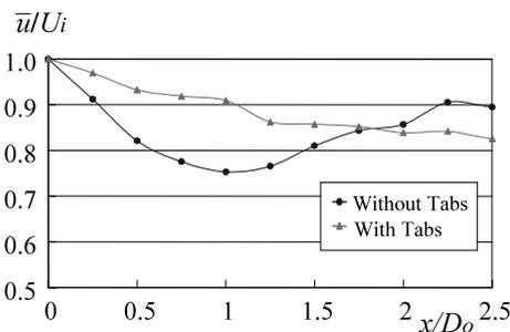
Fig. 7 Variation in axial velocity along centerline for the unexcited jet
