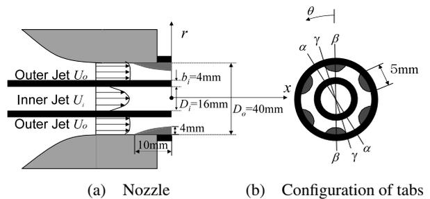
Fig. 2 Schematic diagram of the coaxial nozzle
