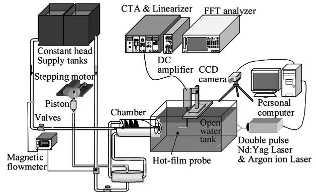
Fig. 1 Schematic sketch of the experiment facility
