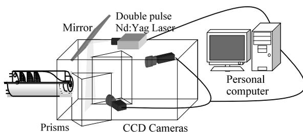
Fig. 3 Schematic diagram of the stereoscopic PIV facility
