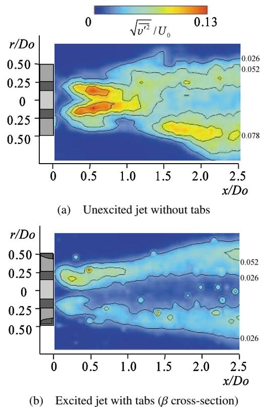
Fig. 14 R.M.S. values of radial velocity fluctuations contours
