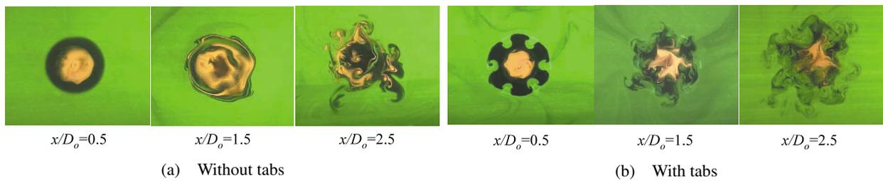
Fig. 5 Visualized flow patterns at  $r$ - $\theta$  cross sections for the unexcited jet
