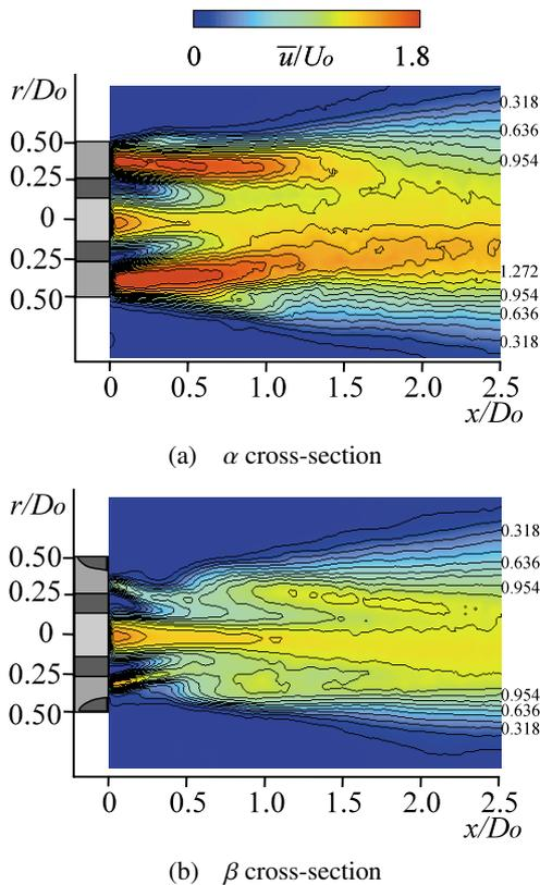
Fig. 13 Mean axial velocity contours for the excited jet with tabs
