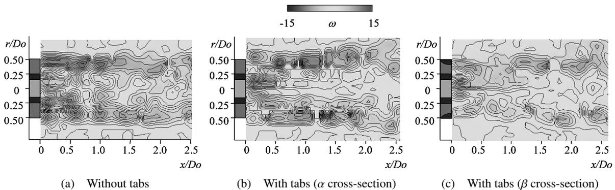
Fig. 9 Instantaneous vorticity contours for the unexcited jet
