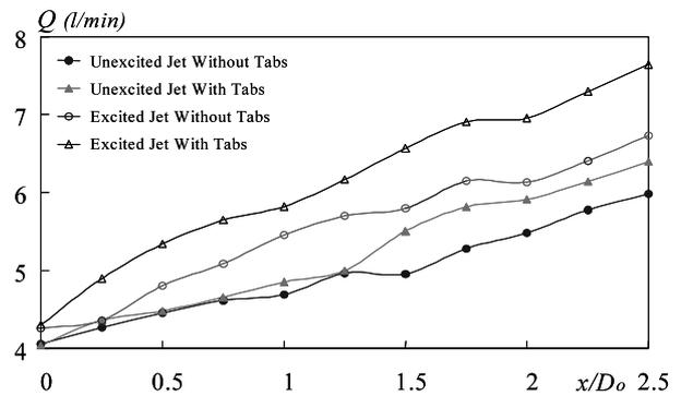
Fig. 18 Streamwise variation in flow rate
