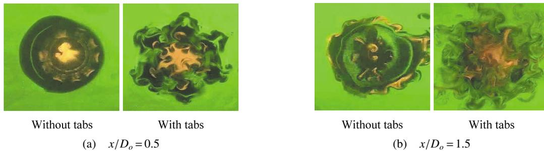
Fig. 12 Visualized flow patterns at  $r$ - $\theta$  cross-sections at  $x/D_o = 0.5$  and  $1.5$  for the excited jet
