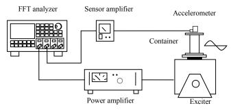
Fig. 1. Experimental setup of size-segregation of grains.
