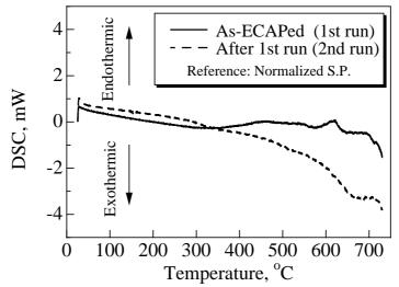
Figure 6. Thermal reaction of as-ECAPed specimen by DSC curve.
