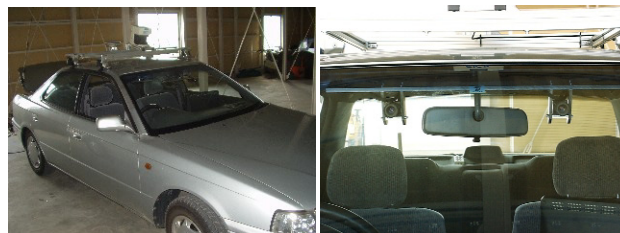
Fig. 1. (a) Overview of our experimental vehicle (Left-side picture). Various measurement sensors are installed in the vehicle such as RTK-GPS, Fiber Optic Gyro, Laser radar, stereovision system, and so on. Furthermore, some actuators are also installed to drive automatically without human. (b) Installation of stereovision system (right-side picture). The stereovision system is installed in front of room mirror.
