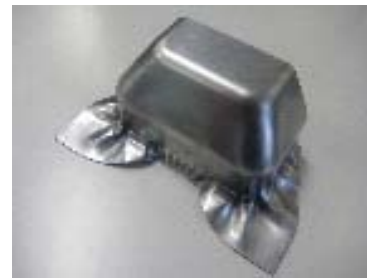
Fig.10 Wrinkling in the experiment
