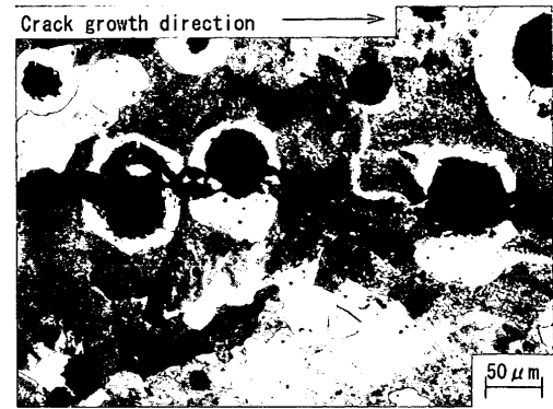
Fig. 6. Optical micrograph of fatigue crack path of SG500 at \Delta K = 9.0 \text{MPa} \sqrt{\text{m}} .
