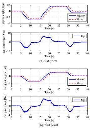
Fig. 9. Time responses in Case 1 (large time delays)
