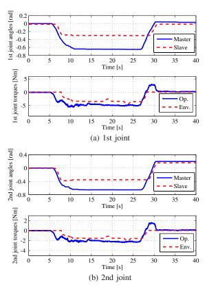
Fig. 8. Time responses in Case 2 (small time delays)
